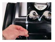
Plug each lamp power wire (white) into the mating connectors on each grav wire (DASH LIGHTS) on the new harness.
